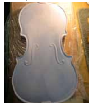
Remove the belly and latex and ease the Styrofoam mould away. The Completed cast! For information please refer to the course notes.
