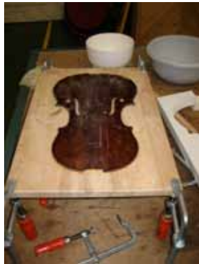
The belly is placed on the base board- if there is any distortion or twist the high edge can be supported with plasticine.
