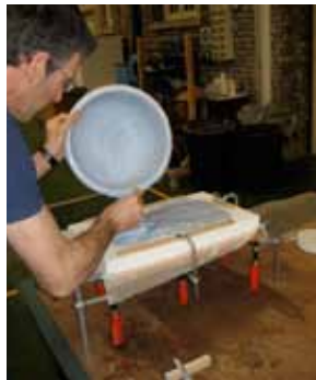
1 kg of plaster is mixed with 3 litres water (approx) and stirred for at least 2 full minutes. The mixing vessel should be tapped several times to remove any air bubbles.
