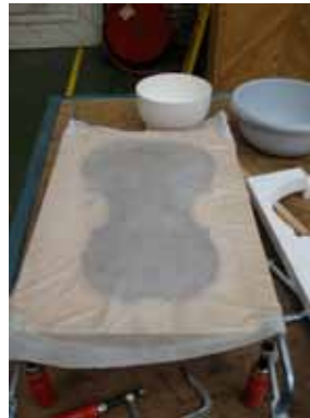
The latex sheet is laid over the belly and pulled tight to avoid wrinkles.
