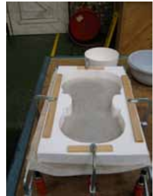
The Styrofoam mould is placed around the belly and Clamped to the base board using blocks to spread the clamping pressure.
