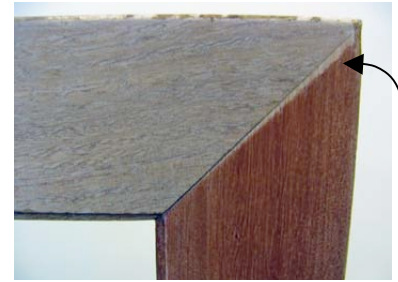
Polyurethane finish over jarrah which has reacted with over stain to form a two part hydrogen peroxide bleach. Note the top horizontal has been treated with a stain initially intended to darken it, the vertical was not treated. See mitre where joints has been taped off
