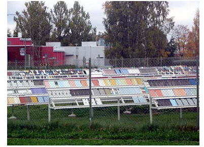
Outside testing panels
