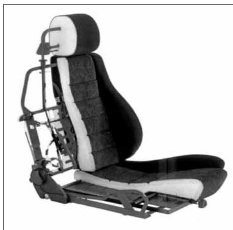
*Steel frame injection moulded foam foundation universally used for motor vehicle seating*
