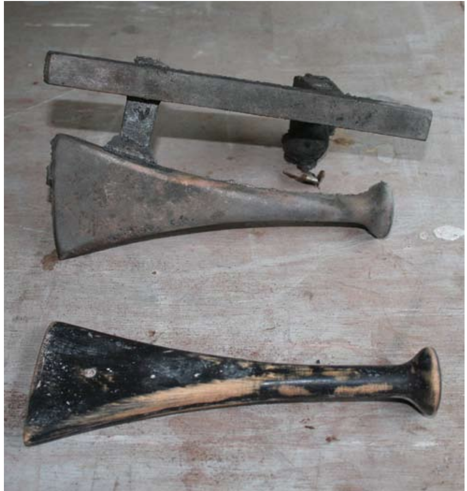
Caulking iron pattern and bronze cast iron
