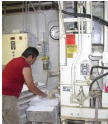
Figure 19: Converted chewing gum machine to make compo
