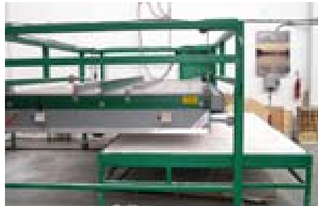
Large kiln with roll away top for firing and slumping architectural glass
