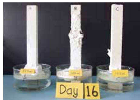
Figure 9. The rate of capillary rise and subsequent evaporation of the solution where the inhibitor has been added is approximately half
