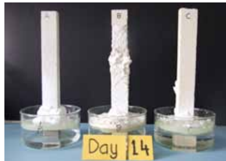
Figure 7. 14 days after contact with the solution and the rupture modulus of the pores of sample B continues to be exceeded by the crystallising salts
