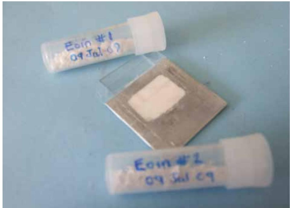
Figure 18. Two vials of the salt samples collected at the Monastery of San Jerónimo and the slide used to hold the samples in position during the analysis process
