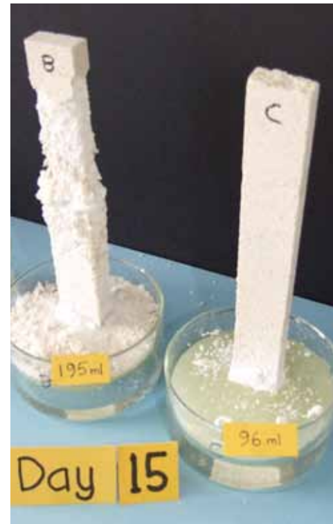
Figure 8. There is extensive damage to sample B on all four sides
