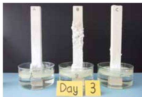
Figure 4. 48 hours after contact and significant crystallisation and some damage is observed on sample B
