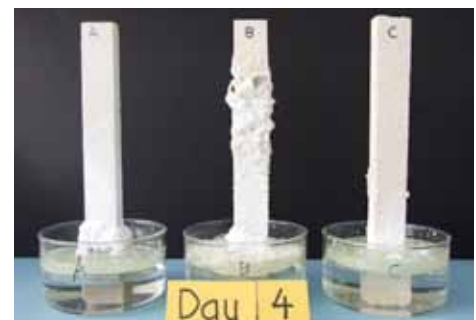
Figure 5. 96 hours after contact with the solution and sample B is experiencing significant material loss
