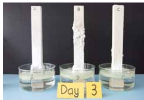
Figure 4. 48 hours after contact and significant crystallisation and some damage is observed on sample B
