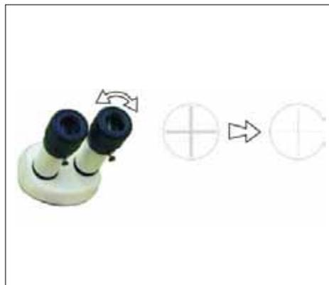
Focusing the Microscope (image courtesy of Rofin Laser Micro)
