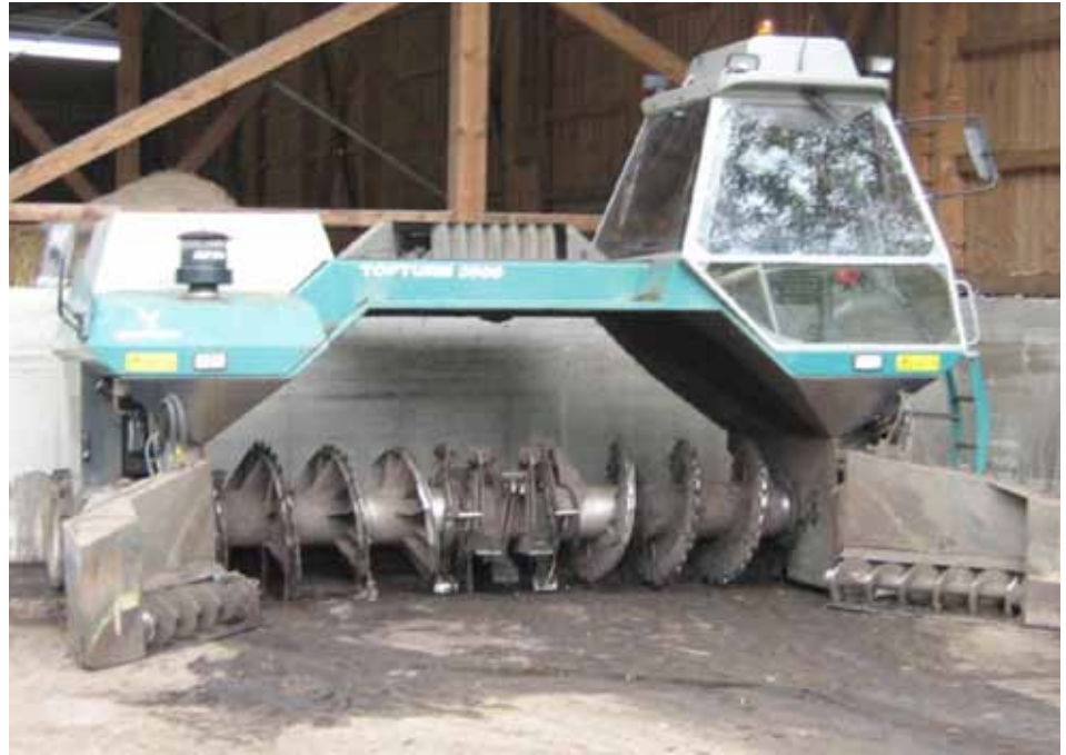
The self-propelled windrow turner—used for mixing and blending—Komptech, Frohnleiten, Austria, June 2009
