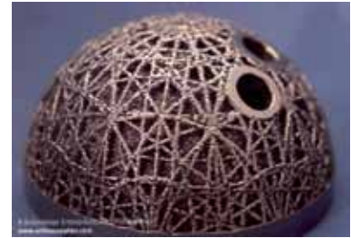
Controlled porosity lattice acetabular cup (Arcam EBM system manufactured by Medical Modelling LLC, Denver)
