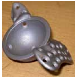
Special design of acetabular cup to suit a damaged hip. Parts displayed by Dr Phil Reeves, Managing Director Econolyst Ltd, Derbyshire, UK.
