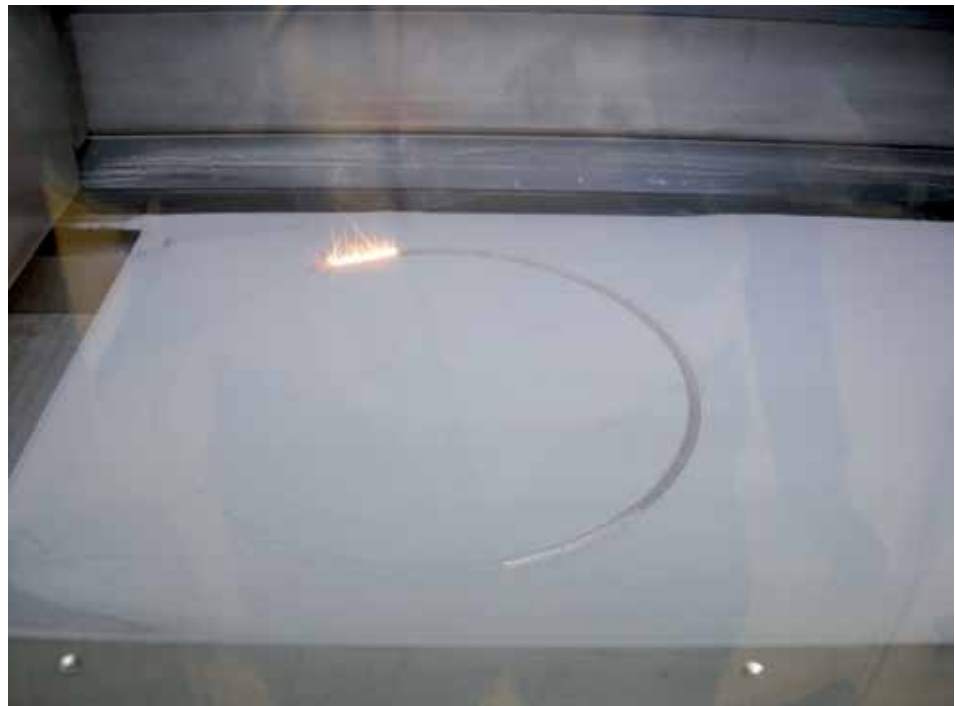
A view of an EOS machine as it sinters the powder at Materials Solutions, the University of Birmingham
