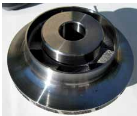
Rocket engine impeller made from Ti6Al4V ELI, weighing 2.5kg. Build time was 16 hours plus machining.
