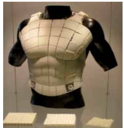
Simulated body armour with spring loaded panels. Designed and manufactured at Loughborough University as a research project.
