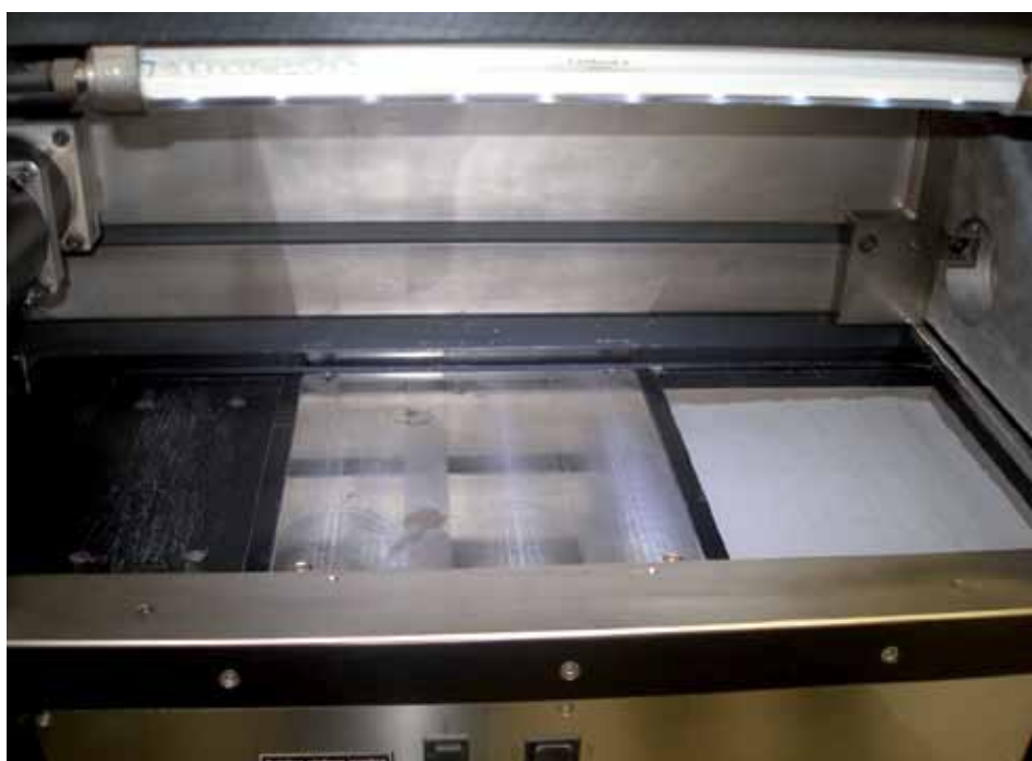
Typical build platform of an EOS SLS RM machine, Materials Solutions, the University of Birmingham
