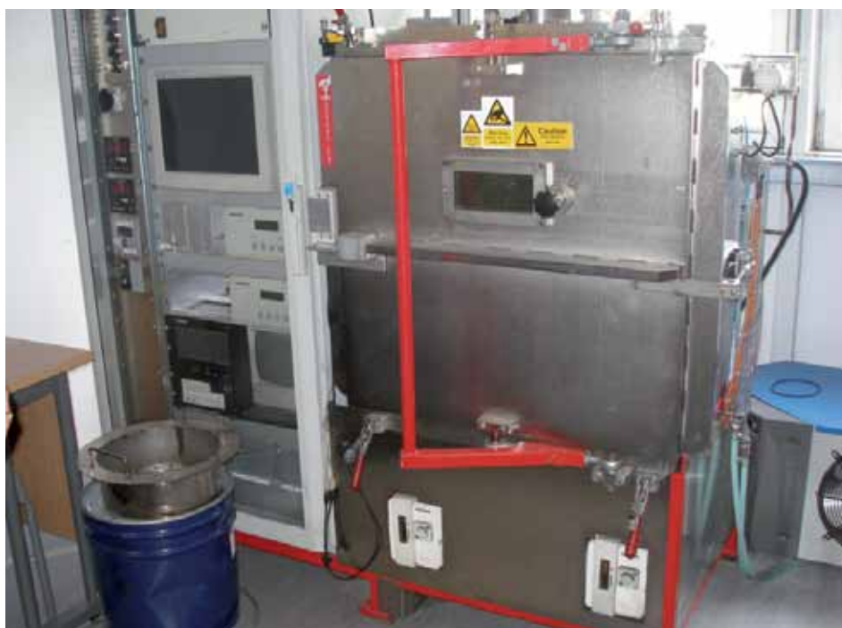
A typical heat treatment furnace as used by the University of Birmingham
