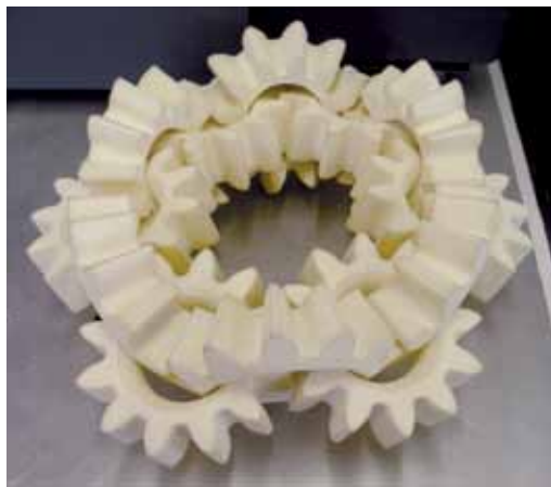
An Impossible design that cannot easily be made in a traditional method. If one gear is rotated, they all rotate. Designed and manufactured at Loughborough University as a research project.
