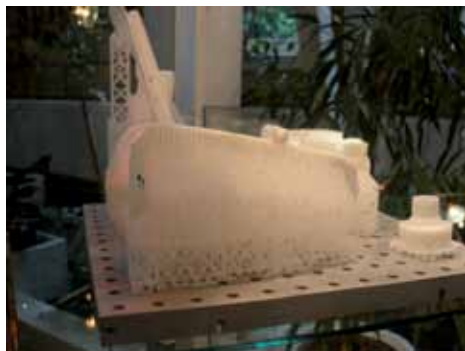
A plastic part with support (Magics software)
