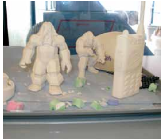
The design of portable radios and action figures. The parts can be made in a couple of hours. If the design is not right, it can be changed and another made.
