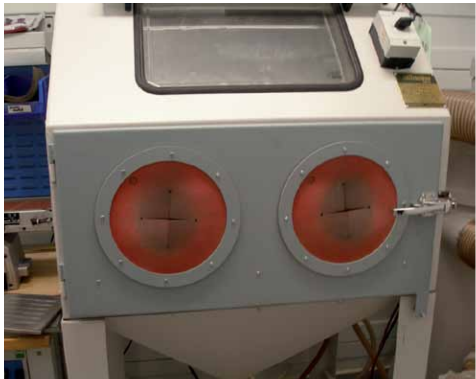
A glove box for high pressure washing of parts after removal from the RM Machine, used at the University of Warwick
