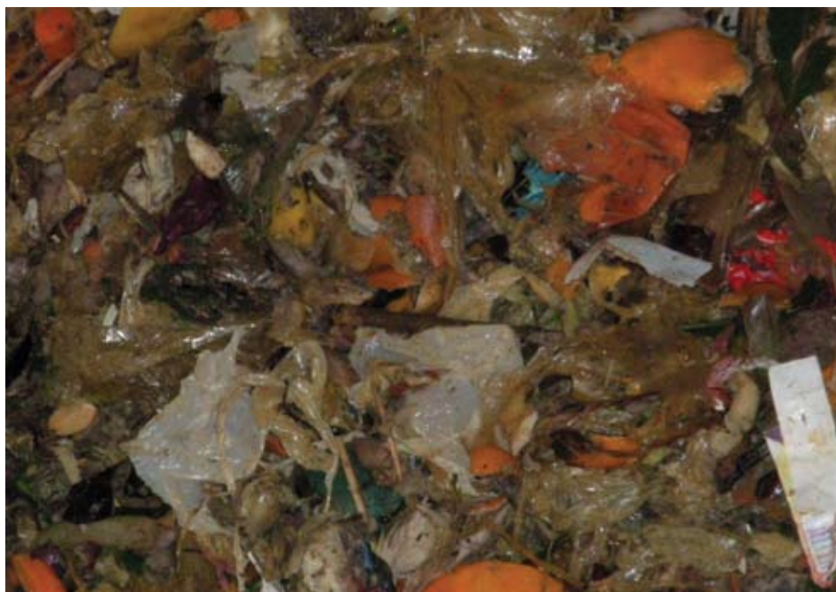
Household and commercial MSW prior to digestion. Note plastic residuals
