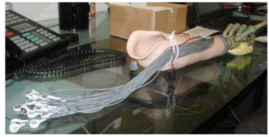
Figure 8: Prosthetic hand with electrodes, showing the various connecting leads from the neuroprosthetic hand to the human brain.
