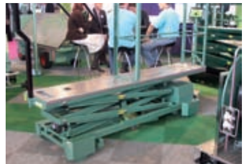
Trolley elevated working platform used on heating pipes
