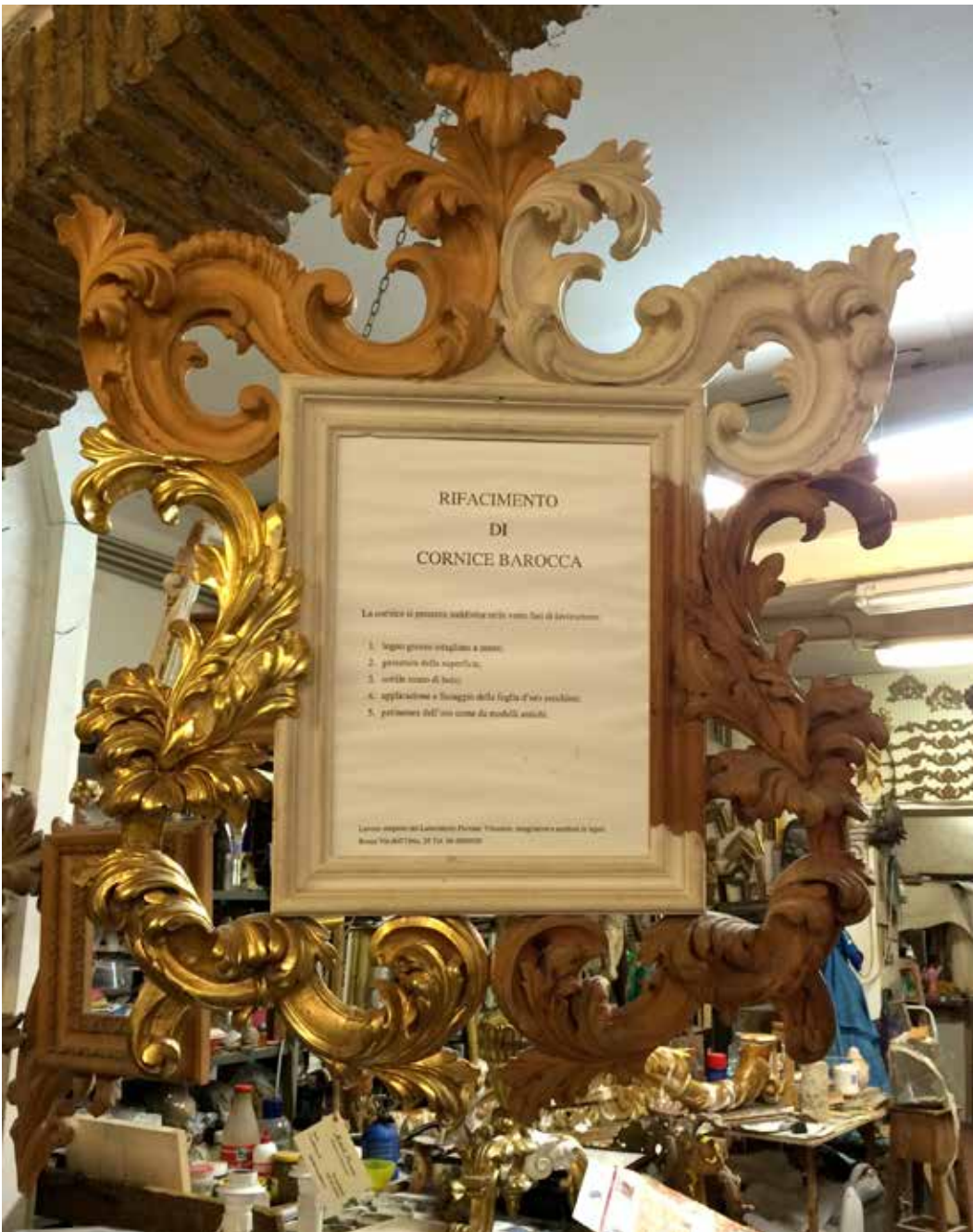
A Baroque-style frame showing the processes involved in woodcarving and water gilding. From the bottom right-hand corner anti-clockwise, we can see the raw carving, the gesso layer, the bole layer and the finished gilded result. Piovono made this frame to illustrate the complexity of the carving and gilding processes to his clients, who were often naive to the skill and complexity of the processes involved in making a frame.
