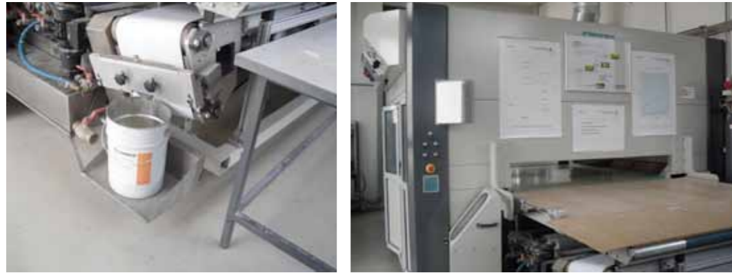
Recovery belt for waste recover on CNC spraying machine
