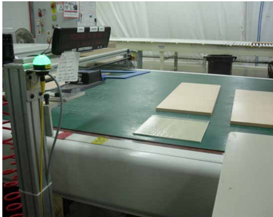
Chip scanner for CNC spray line
