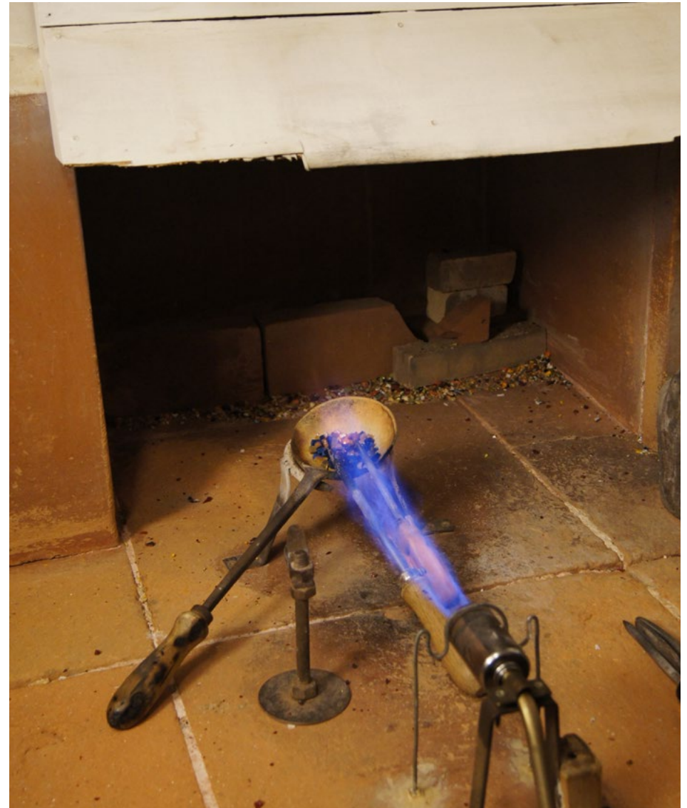
Glass being melted together in crucible to create custom colours and textures for mosaic images
