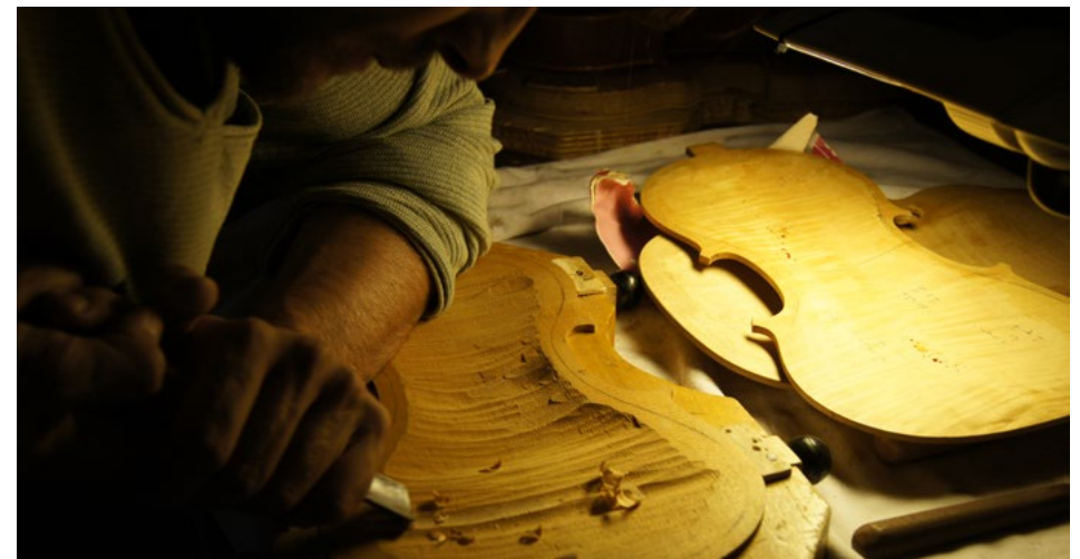
Roberto Cavagnoli demonstrates using a gouge to hollow out the inside face of the violin
