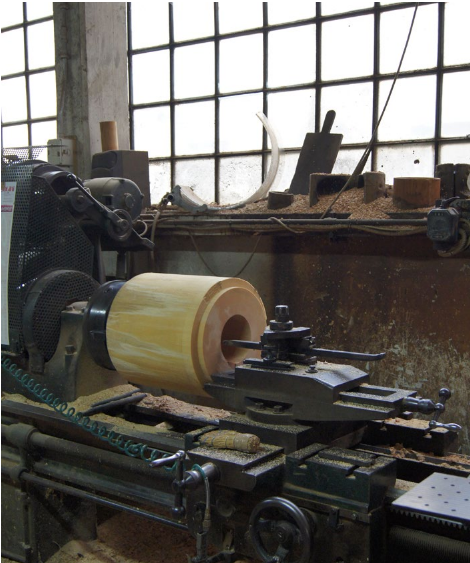
Arcangeli brothers further refine the internal shape of the mold using custom workshop made tooling specific to each mold profile
