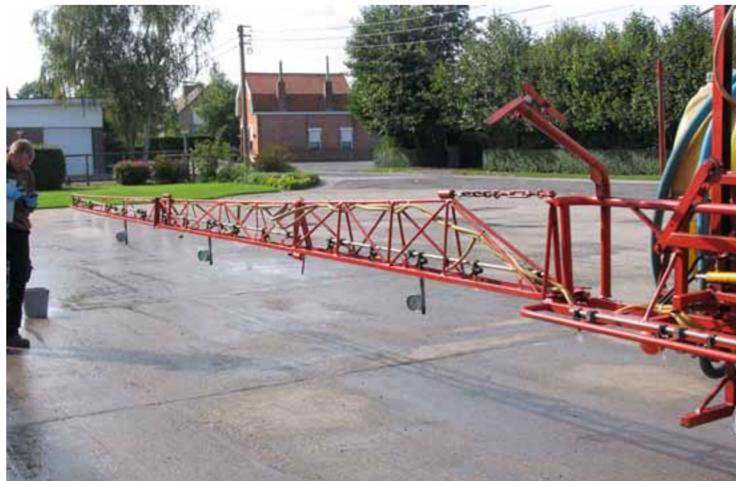
Testing boom line pressure at a mobile testing station located in the Flanders region
