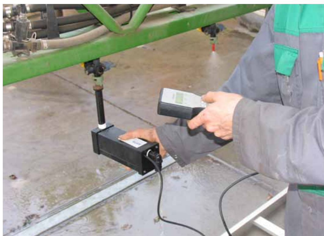
Testing of individual nozzles with a computerised flow meter in the Netherlands
