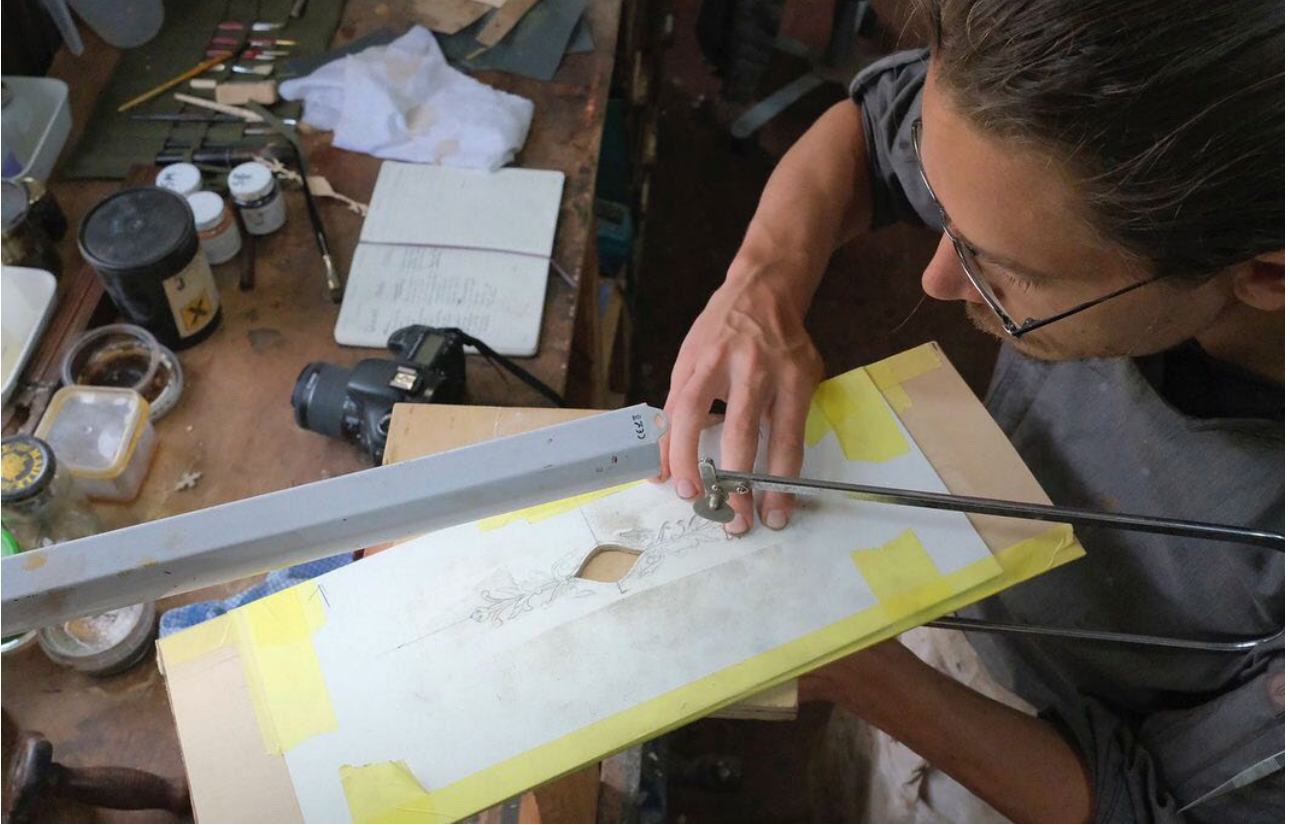
Figure 12. Cutting the marquetry for the replacement lid using traditional techniques.
