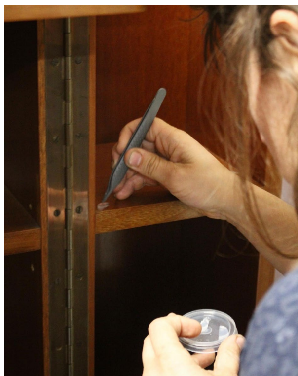
Figure 5. Marine Prevet applying agar gel sample to interior surface of 20th century cabinet in order to test surface ph and conductivity.
