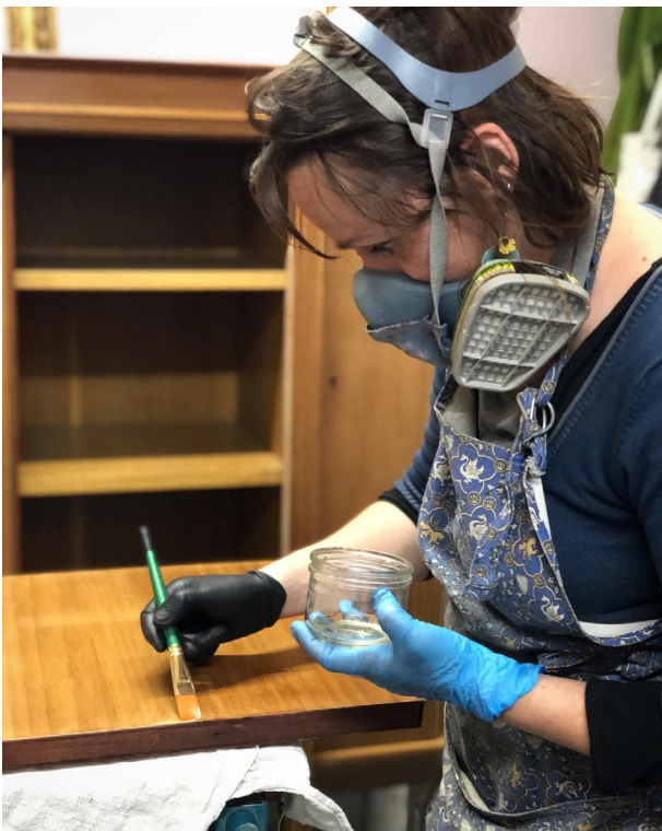
Figure 18. Marine Prevet regenerating a Nitrocellulose based finish with solvent mixture.
