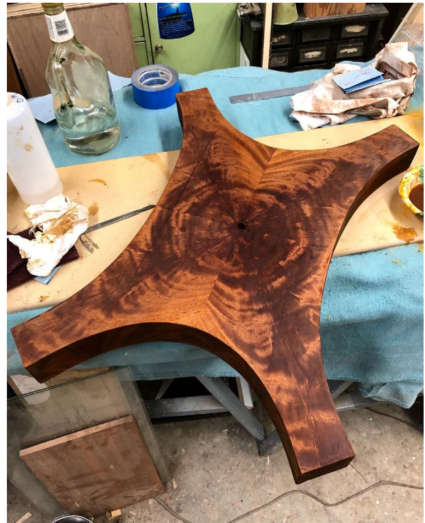
Figure 10. Empire table base with quartered mahogany crotch veneer after being applied with traditional hammer veneering technique.
