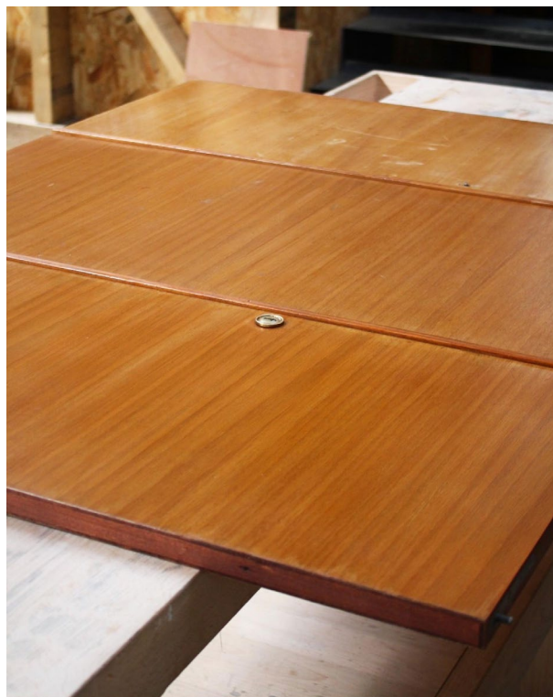
Figure 19. Comparing results of nitrocellulose regeneration process by Marine Prevet. The farthest panel is pre-treatment, and the nearest panel is post treatment.
