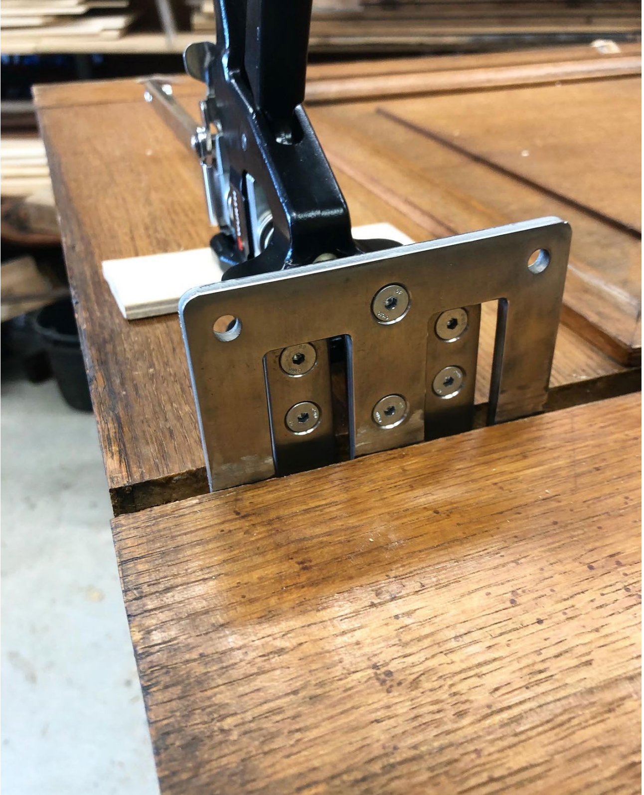
Figure 4. Carefully disassembling the Teylers Museum door in the Bruijs en Streep workshop using a shop modified tool.
