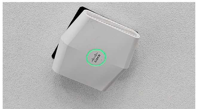
Figure 12: Image of a Cisco smart sensor measuring Co2, vaping smoke, and other air quality metrics
