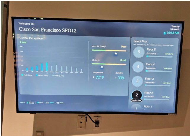
Figure 2: Image of Cisco spaces app on a TV screen. This shows key information at a glance, such as occupancy levels per floor, air quality and Co2 levels throughout the building.
