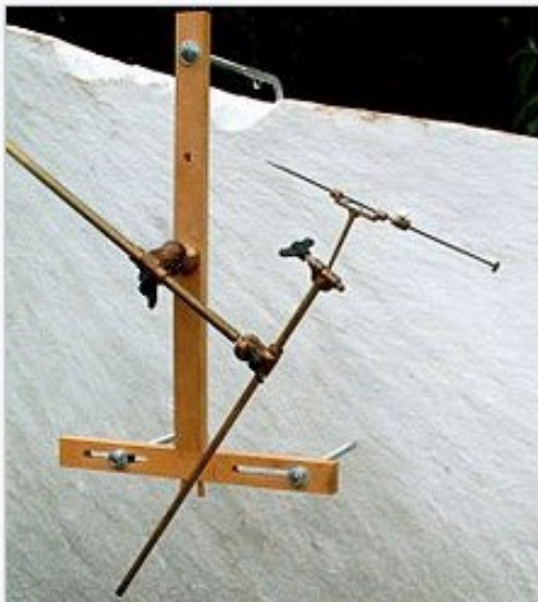
La macchineta di punta, employed to make accurate reproductions (photo credit Wikipedia)
