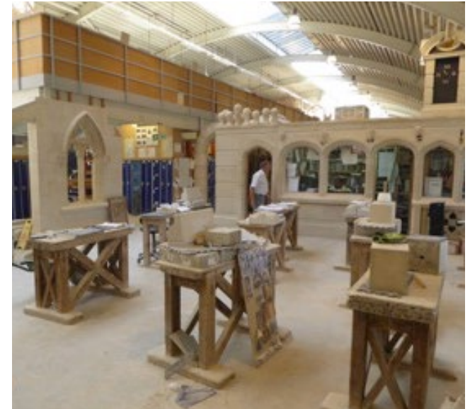
The stonemason's work station, the banker
