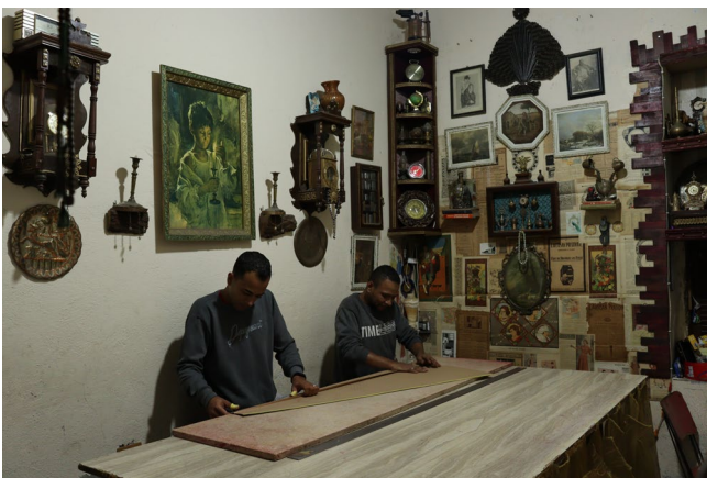
Figure 55. Walid and Shady prepare the radial folds of a sunray mould
