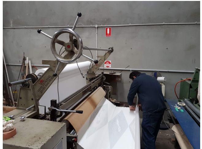
Figure 24. Simon feeds fabric between the protective tissue paper before it is pleated
