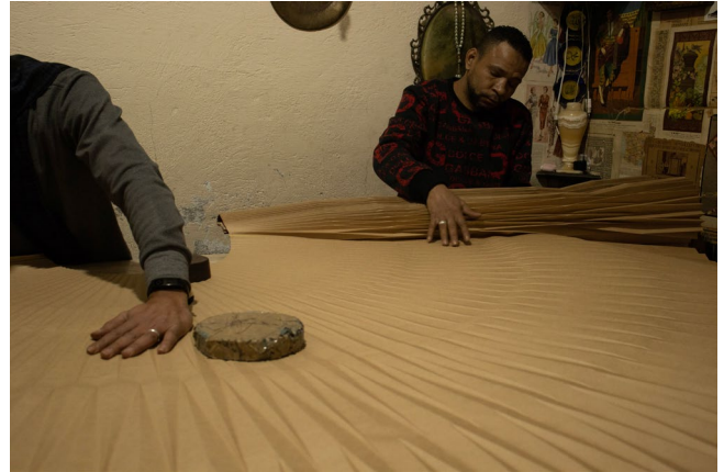
Figure 16. The top layer of the mould is rolled back
