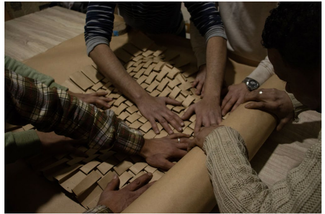
Figure 66. A basket weave mould is pushed in four directions requiring many hands
