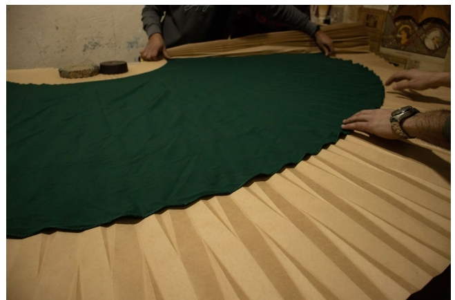
Figure 18. The fabric is laid out in position across the mould
