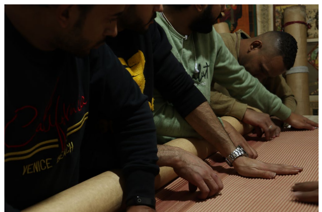
Figure 68. A 5m mould of 5mm accordion pleats is prepared for steaming
