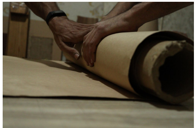
Figure 67. The mould is rolled in between a sheet of card before steaming
