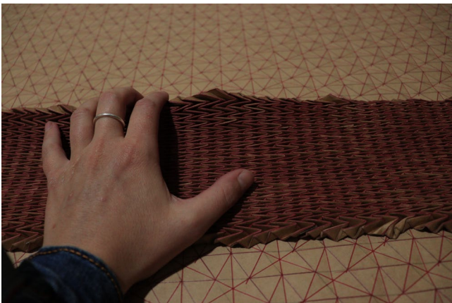
Figure 52. Collected chevron mould resting on top of unfolded three point star pattern (aka Mercedes)
