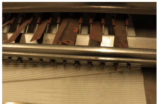
Figure 4. Damaged pattern cards
