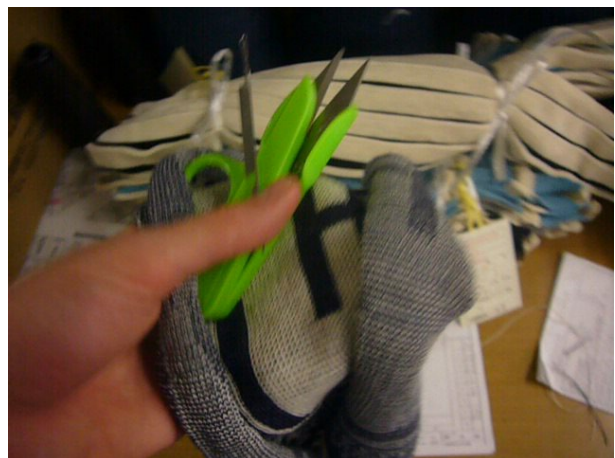
Figure 32. Repairing tools; snips and a machine needle for tucking in stitches
