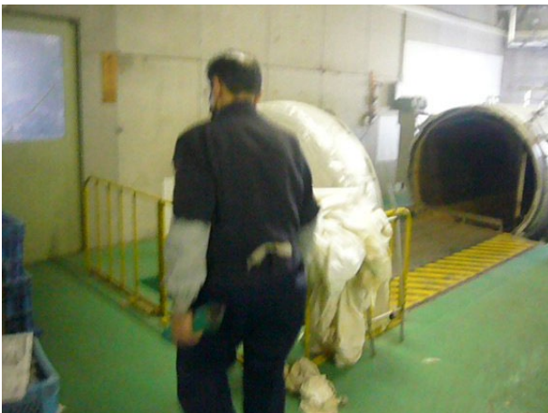
Figure 50. The steaming chamber that large crates of bobbins are put into after spinning
