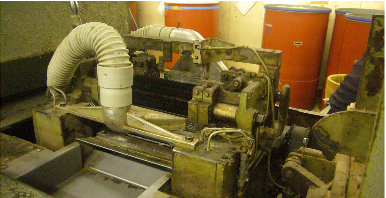
Figure 8. Combing box that contains rows of combing needles of the High-speed Giller
