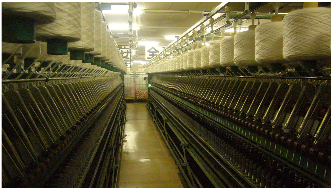
Figure 13. The many heads of spindles and heads of wool on a ring spin machine
