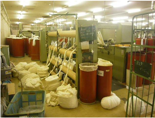
Figure 38. Mixing machine from the back and front. Intake rollers and splicing trays
