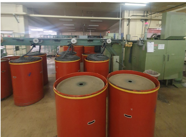
Figure 39. Leveller side profile, intake rollers and knot spreader
