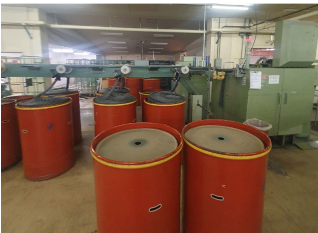
Figure 7. Leveller side profile, intake rollers and knot spreader
