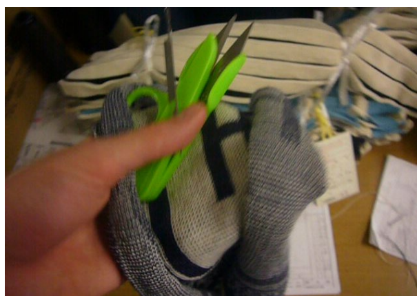
Figure 64. Repairing tools; snips and a machine needle for tucking in stitches
