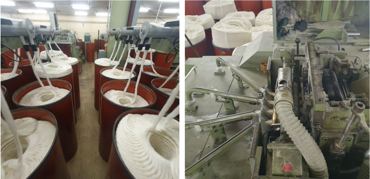
Figure 10. The numerous cans being fed into the rubber and its quad output
