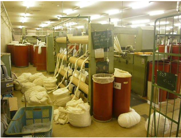
Figure 6. Mixing machine from the back and front. Intake rollers and splicing trays
