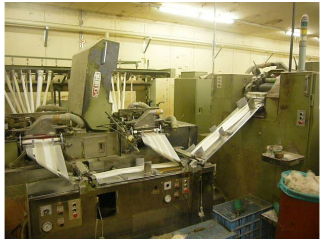
Figure 6. Mixing machine from the back and front. Intake rollers and splicing trays
