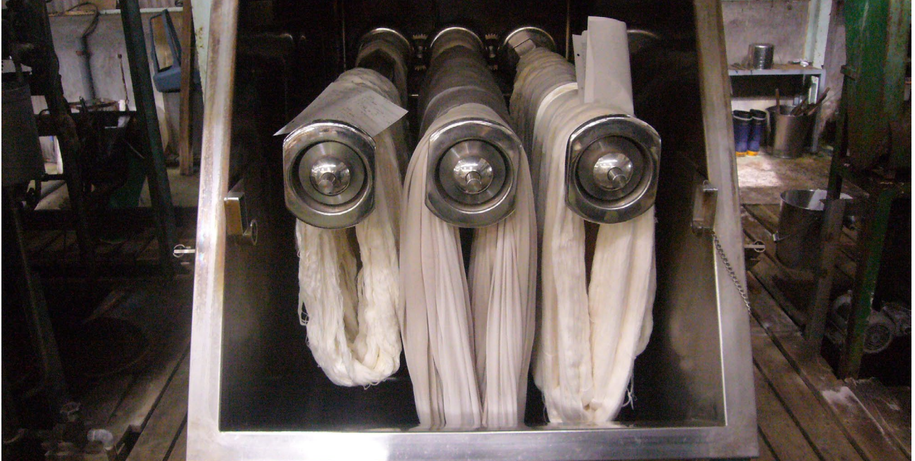
Figure 53. A closer look at the hanks, hanging on rails in the dye vat.
