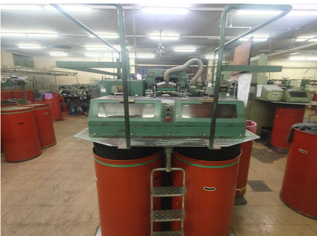
Figure 9. The twin cans of the Bi-coiler
