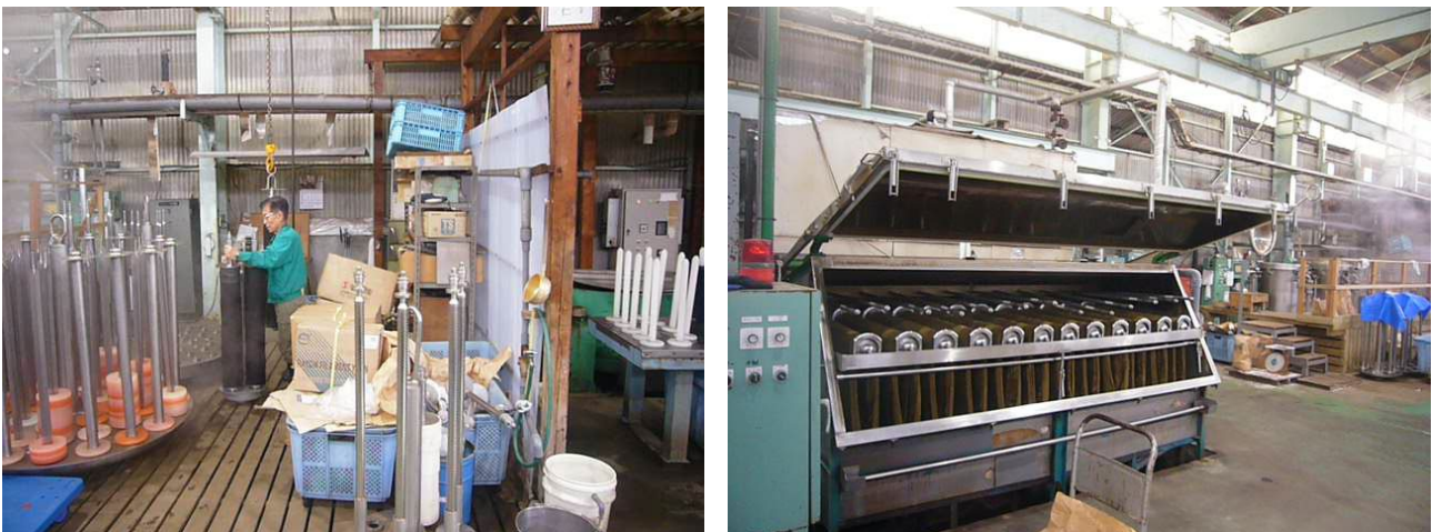
Figure 52. Left, cheese dyeing. Right, hank dyeing
