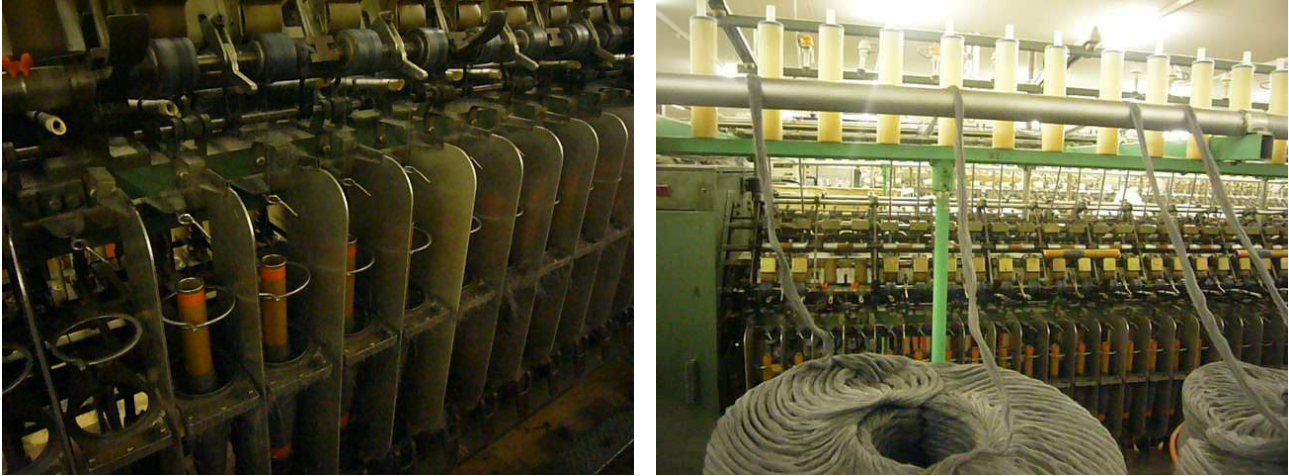
Figure 47. The chunkier knitting yarn ring spin machines
