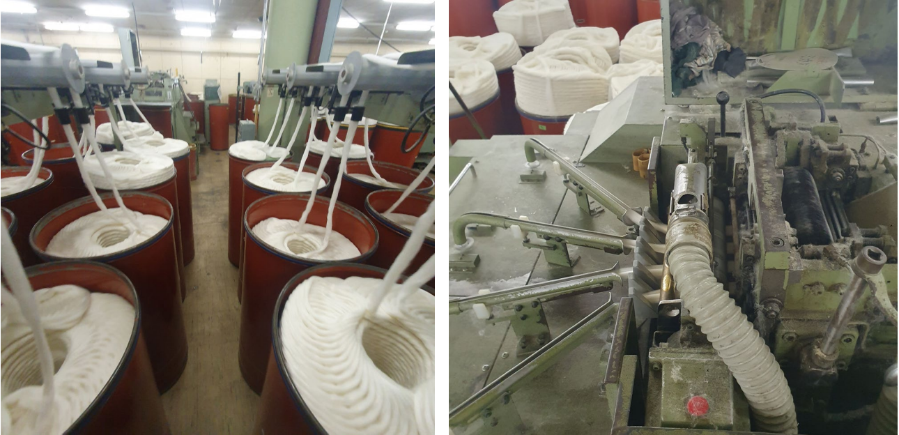
Figure 42. The numerous cans being fed into the rubber and its quad output
