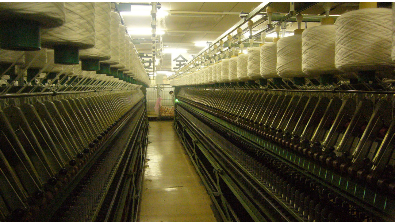
Figure 45. The many heads of spindles and heads of wool on a ring spin machine
