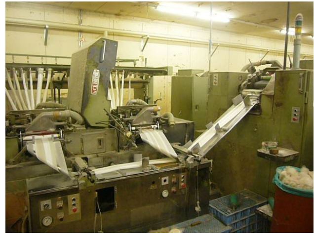
Figure 38. Mixing machine from the back and front. Intake rollers and splicing trays
