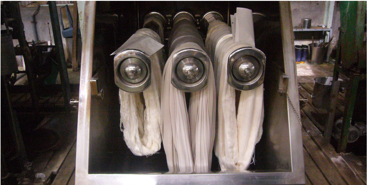
Figure 21. A closer look at the hanks, hanging on rails in the dye vat.
