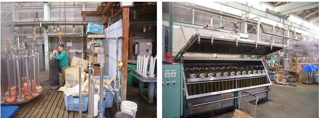
Figure 20. Left, cheese dyeing. Right, hank dyeing
