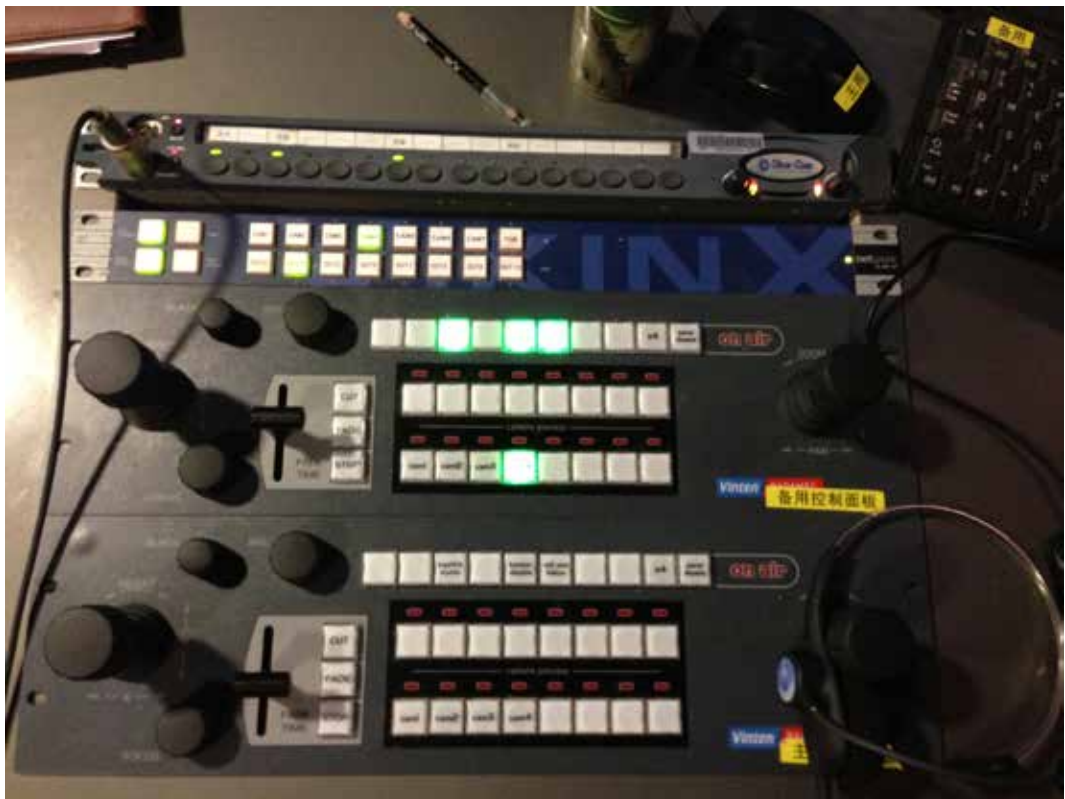
SMG Dragon Robotic camera control made by Vinton
