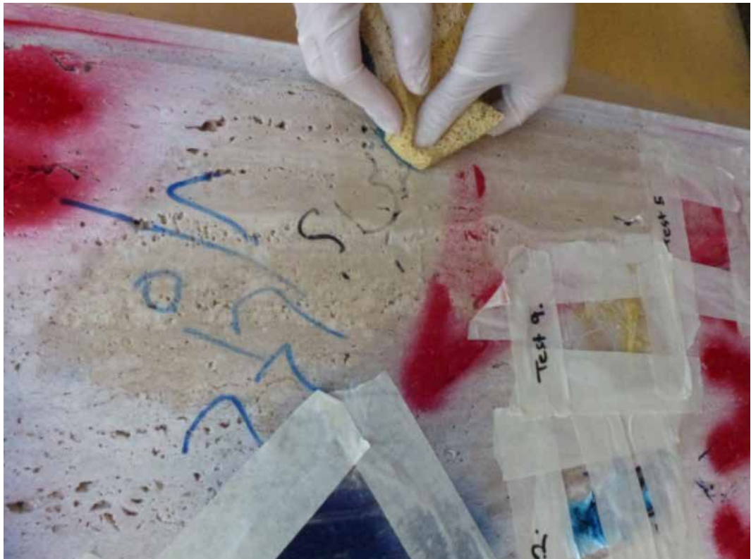
Testing graffiti removal materials and methods
