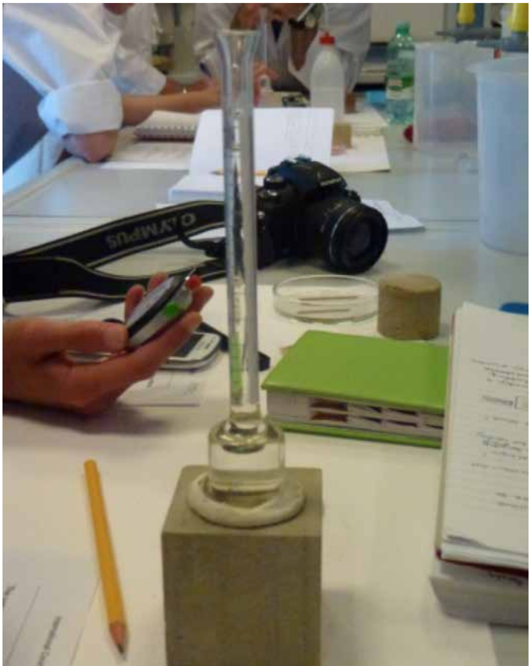
Measuring the porosity of stone, ICCROM labs
