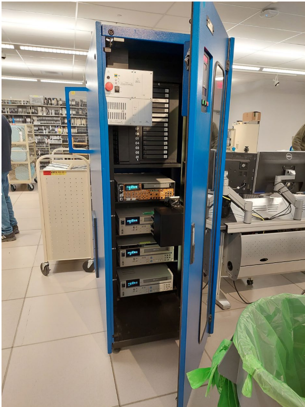
Figure 12. A SAMMA robot for VHS massed digitisation
