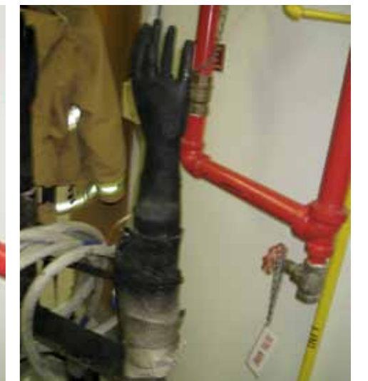
The burns sustained by the PyroHands Fire Test System after the test has been conducted
