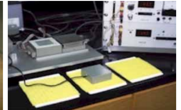
The fabric sample going through the warm-cool touch testing process
