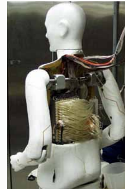
The NCSU's Advanced Sweating Thermal Manikin, Coppelius
