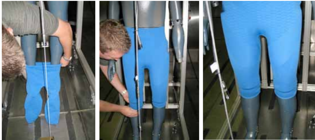
These three images show the dressing of the Advanced Sweating Thermal Manikin in a garment ready for testing
