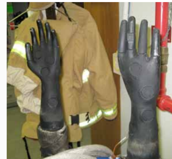
The PyroHands Fire Test System used to test protective glove prototypes
