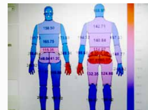
A diagram illustrating the different sections of an Advanced Sweating Thermal Manikin
