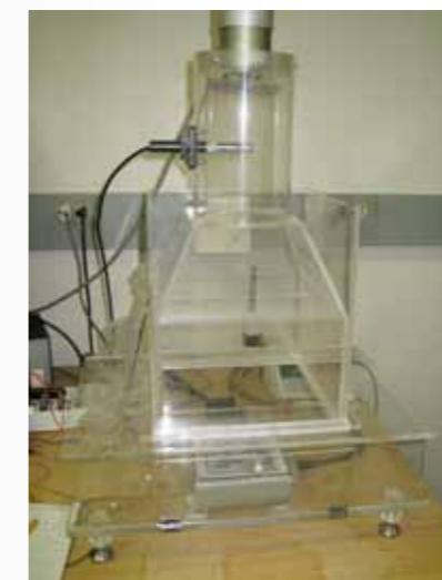
The Cooling Ability/Breathability Test using the KESF-TL-2C
