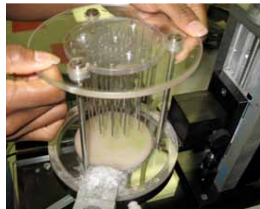
Lifting the glass plate for the insertion of the fabric sample
