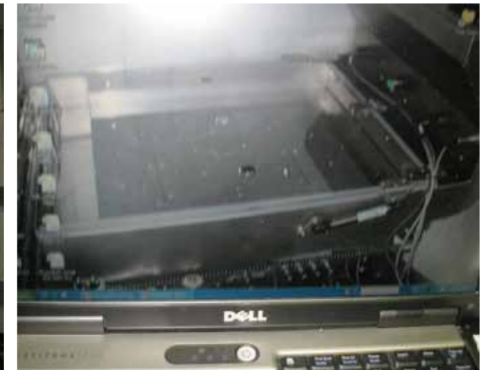
The Cooling Ability/Breathability Test using the KESF-TL-2D Large Hot Plate
