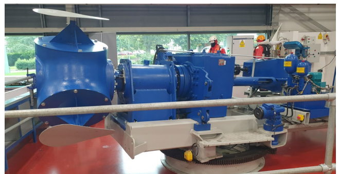
Figure 17. Large scale simulated nacelle with working componentry
