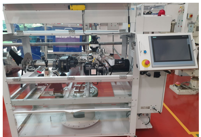
Figure 18. Festo Nacelle Simulation Tool with Siemens Gamesa Operating System which is fully programmable for the purposes of fault simulation.
